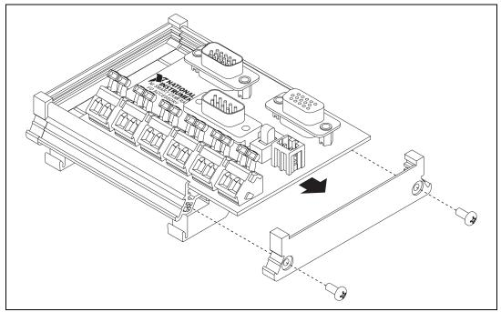
Figure 4. Removing the Circuit Board
